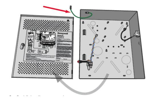
2. Partially install the four power supply screws.
